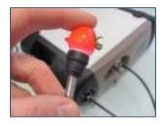
Using a near infra-red portable spectrometer, the lab has expertise in screening hundreds of fruit per day for at least the six following parameters: color Hue, color Chroma, juice soluble solid content, juice pH, firmness and water content. More developments can be initiated for the prediction of additional quality parameters of the fruit and other plant organs.
